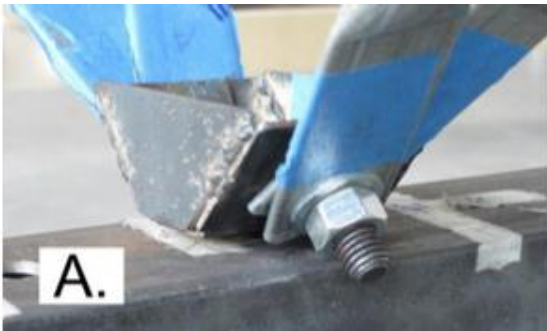
Early truss node prototype to identify efficient, low cost web connection options!
