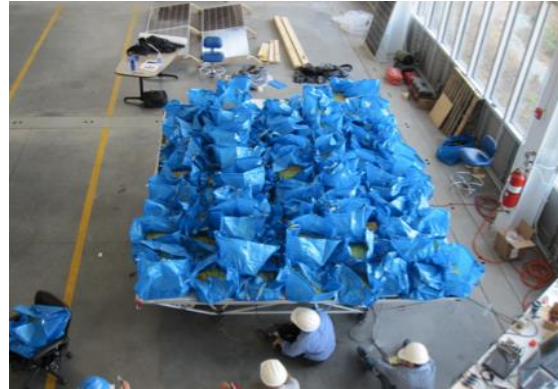
Physical load testing performed to validate structural integrity of prototype QuadPod!
