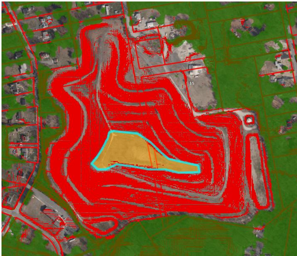
Figure 3 – Oak Avenue Rubble Landfill with 10% or greater slopes shown in red, and suitable solar acreage shown within the blue outline.
