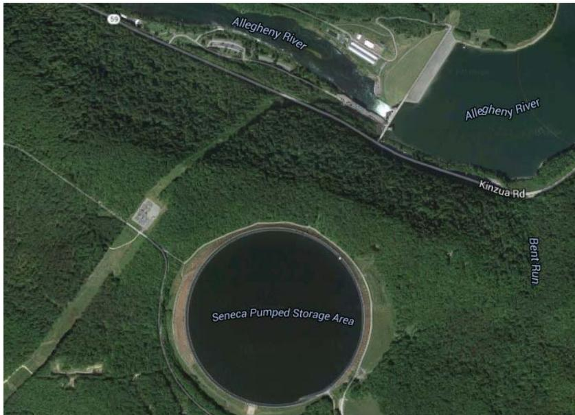
Owned by FirstEnergy, the Seneca Pumped Storage Generating Station functions like a battery. It absorbs excess power generated by plants such as FirstEnergy nuclear and fossil-fuel fired baseload plants in off-peak hours, such as nighttime, using it to pump water into a reservoir. Later, when demand exceeds the base load, the flow of water from the reservoir generates additional electrical power to meet peak load demands.
